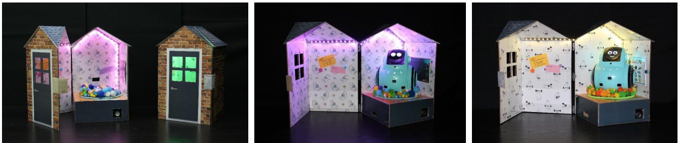
Figure 1: Illustration of interactive product packaging for child-robot interactions: Through co-design sessions with children, we developed a box with a social entity to guide initial interactions with social robots during the “unboxing” of the robot. The box was designed with aesthetic features to support a narrative for the box and robot, including both verbal and non-verbal communicative features to socially engage with the children. While serving as a “home”, the box supported and facilitated the initial child-robot interaction, by providing introductions of the robot and instructions for initial ice-breaker activities.
